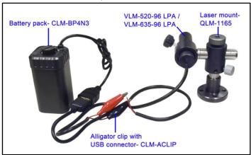
1. Insert the laser module into the holder and tighten the screws to securely fix the laser module onto the mount.
