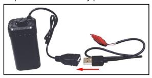
3. Clip the red alligator clip to the red lead of the laser module and the black alligator clip to the black lead to power on the laser module.
